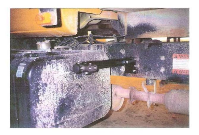
Next you need to put a  $\frac{1}{2}$ " return port into the hydraulic tank. On the top side of the tank locate the area that is away from any outlet ports. Drill a  $\frac{1}{2}$ " hole in the tank. Weld in place the  $\frac{1}{2}$ " elbow provided in the kit.
