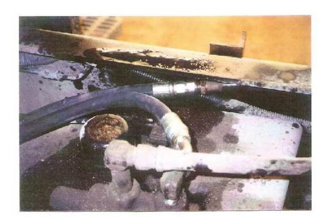
Pump to diverter valve. Hose connection to the pump (port "C" on diverter valve)
