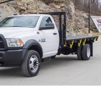
MODEL : PCT9612 - 3/16 12' X 96" STRUCTURE LINE PLATFORM 3/16" TREADPLATE FLOOR 4" STRUCTURAL CHANNEL CROSSMEMBERS ON 12" CENTERS 6" STRUCTURAL CHANNEL SIDE & END RAILS 6" STRUCTURAL CHANNEL LONGSILLS 1/4" OUTSIDE POCKETS W/ 3/8" X 2" RUB RAIL SLIDING WINCH TRACK FULL LENGTH ON DRIVERS SIDE 5EA SLIDING WINCHES W/ 4" X 27' STRAP W/ FLAT HOOK 1EA WINCH BAR PAINT BLACK
