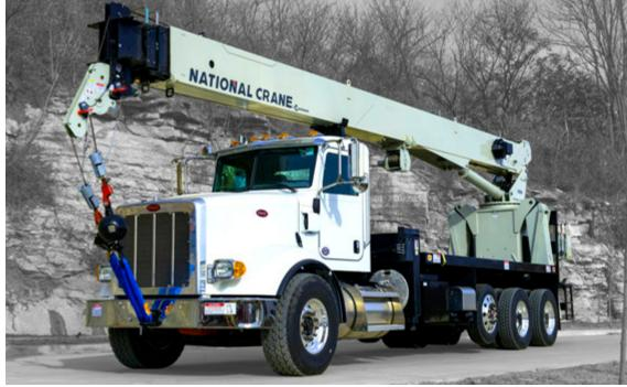
26-TON RATING 125' (4 SECTION) BOOM REAR MOUNT INSTALLATION DUAL CONTROL STATIONS HYDRAULIC CAPACITY ALERT WITH INTERNAL WIRE A28 (ANTI 2 BLOCK) BURST-OF-SPEED WINCH 375° NON. CONTINUOUS ROTATION 18' STEEL FLATBED A-FRAME MAIN OUTRIGGERS OUT/DOWN AUX OUTRIGGERS - MOUNTED OVER FRAME CENTER REAR OUTRIGGER 9/16" ROTATION RESISTANT ROPE LOAD BILL W/SWIVEL HOOK **1 SHEAVE LOAD BLOCK** TRIPLE PUMP HYDRAULICS HOT SHIFT PTO
