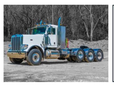
AIR SLIDE 5TH WHEEL AIR & ELECTRIC LINES (COILED) COLLECTED ON HOSETENNA 7-WAY PLUG 1/4 FENDERS ON REAR TANDEM AXLES
