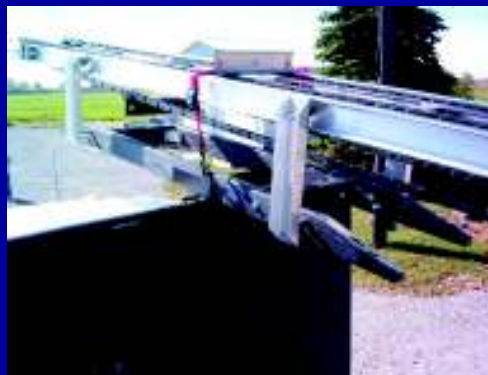
Step 2 Swing unit out to side or rear of truck bed and level.
